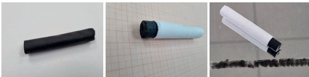
Fig.1 Soil type B is formed into a pin (left), wrapped with a paper/foil (middle), and applied in stripes onto the mirror tile (right) (image source: SONAX GmbH).
