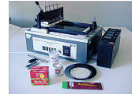
Fig. 3 Equipment to perform the cleaning performance test.
